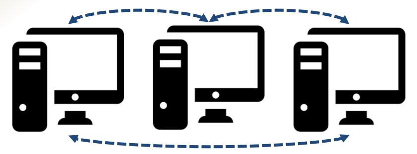
Multiple individual computers linked together using a fast communication network
